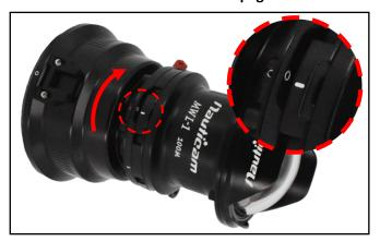
Turn the lens clockwise until the "I" mark on the lens aligns with the WHITE dot on the converter and a "click" sound is heard.
